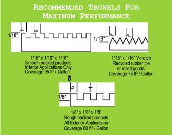
Trovel size is suggested to maximize coverage of achesive. Periodically check coverage of achesive during installation. Uneven sub flooring may require the use of either a leveling/patching material, or a larger noticed trovel for proper coverage of achesive. Always refer to the flooring manufacturer's recommended use instructions for proper trovel selection.
